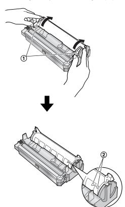
**6** Remove the used cartridge (1) from the drum unit (2).
